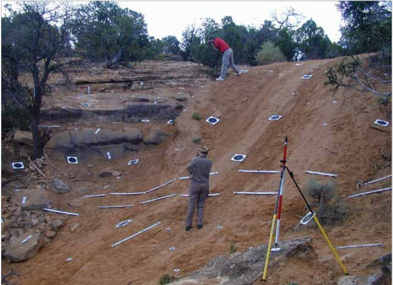
BLM geographer Neffra Matthews (bottom) and BLM physical scientist Tom Noble take a series of photos so they can use close-range photogrammetry methods to create three dimensional surface information to help quantify effects from rapidly increasing off-highway vehicle (OHV) use in the Dry Creek Extreme OHV Area.
